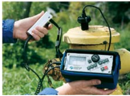
Leak Surveying by listening at a hydrant with magnet base
