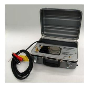
The 3020 Compressor is a useful option for low-flow sampling of wells at depths to 200 feet. It runs on a 12 volt DC electrical supply, and can be connected to your vehicle's battery with the supplied cables, or driven by a separate power source. At just 15x11x6-1/2" and 15 pounds, it offers an extremely convenient, portable pneumatic power choice for many sampling systems.
