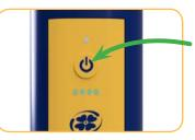
Hold the Power button down until the bottom LEDs flash back and forth and then turn off.
