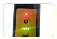
The device lights will turn on and blink according to charge level.
