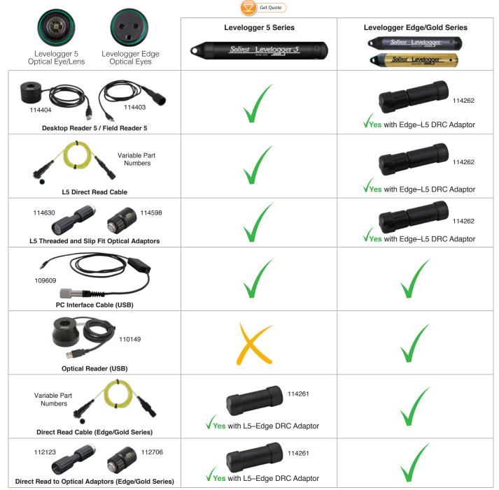
\*Using an L5-Edge DRC Adaptor with an older style optical reader will allow programming and diagnostic reporting, however, it will not allow data downloading from a 5 Series datalogger. In this case, a Desktop Reader 5 or Field Reader 5 must be used.
