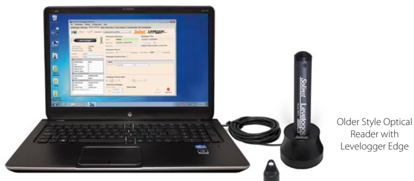
Figure 2-5 Levellogger Edge Connected to a PC Using an Older Style Optical Reader
