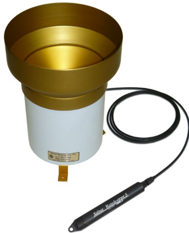
Figure 10-21 Rainlogger 5 Connected to Tipping-bucket
