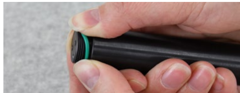
Figure 10-26 Replacing Levellogger O-rings
