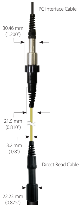
Figure 10-8 L5 Direct Read Cable Dimensions
