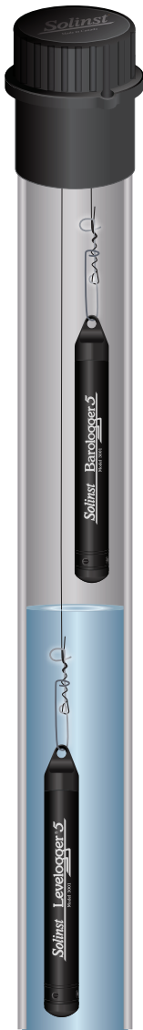
Figure 10-18 Levellogger and Barologger in Well
